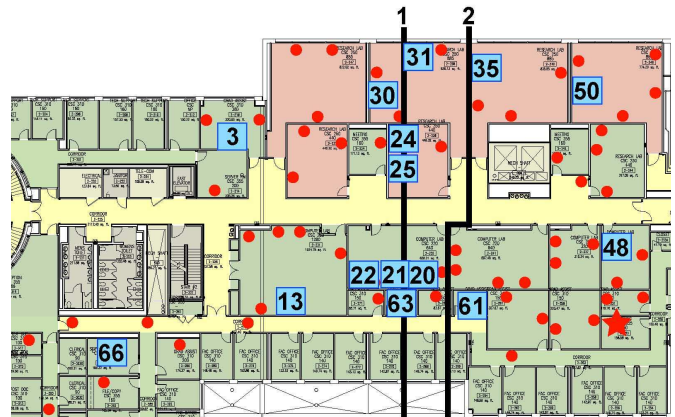
Figure 1. The WiSeNet testbed (73 MicaZ motes; 152.5 feet \times 97 feet).
