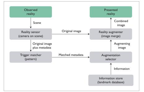
Figure 3. Conceptual architecture of an augmented reality app. An AR app resides on the path from reality as observed to reality as presented (with augmentations) to a user. It involves determining the relevant part of the reality, finding whether and how to augment it, and then inserting the augmentation and presenting the augmented view to a user.
