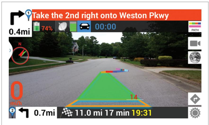
Figure 1. Augmented reality GPS Drive/Walk Navigation app. The app augments the user’s view of reality with the suggested path, indicating the distance to the next turn.
