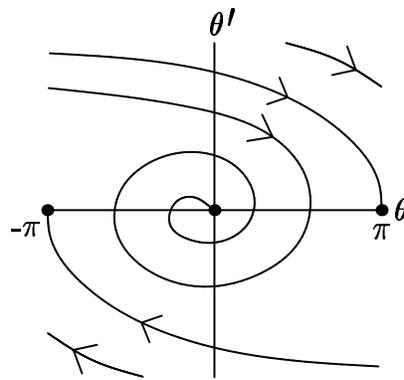
Figure 3: Phase diagram for the damped pendulum.
