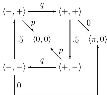
Figure 8: Prototypical transition probabilities for the pendulum with  $q = (1 - p)/2$ . Self-loop probabilities are not shown.
