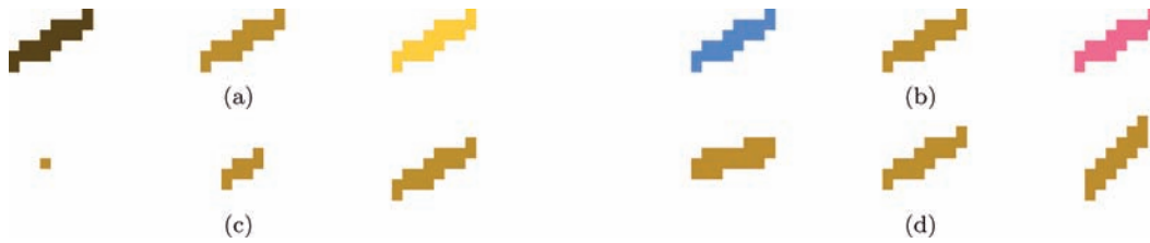
Fig. 3. Visual features used during the resolution experiment; all elements shown at 8 \times 2 resolution except for size feature: (a) dark, medium, and bright luminance, CIE xyY = (0.44, 0.48, 6.7), (0.43, 0.48, 13.6), (0.38, 0.43, 19.5) , respectively; (b) blue, brown, and pink hue, CIE xyY = (0.22, 0.23, 13.7), (0.43, 0.48, 13.6), (0.34, 0.28, 13.6) , respectively; (c) 1, 4, and 16 pixel size; (d) 15^\circ, 35^\circ , and 55^\circ orientations counterclockwise from horizontal.
