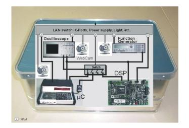
Figure 3. A remote lab-in-a-box for embedded applications.
