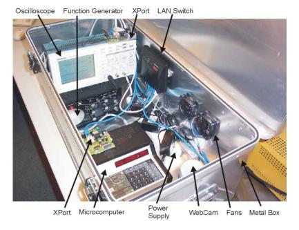
Figure 4. Test installation of the lab-in-a-box.
