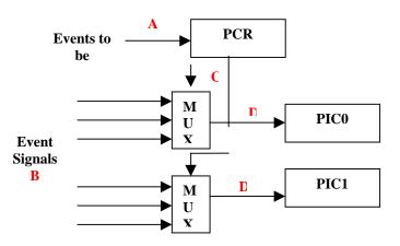
Figure 2 The PCR control signal determines which event will increment the PIC
