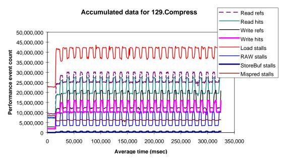
Figure 1 UltraSPARC Performance Data from 129.compress (SPEC95)
