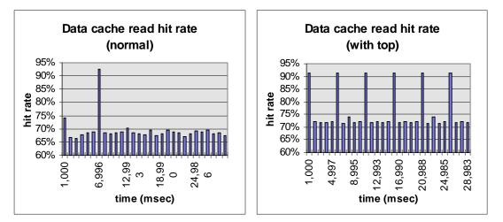
Figure 4: The Data cache read hits without top running and with top running
