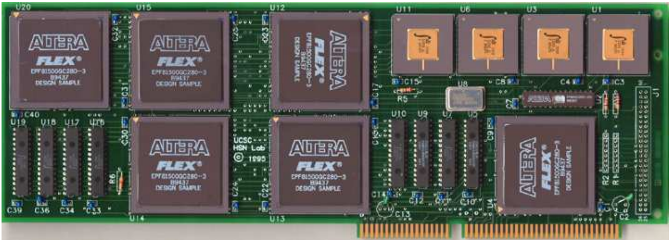
Fig. 1. The CPU Design Kit prototyping board.
