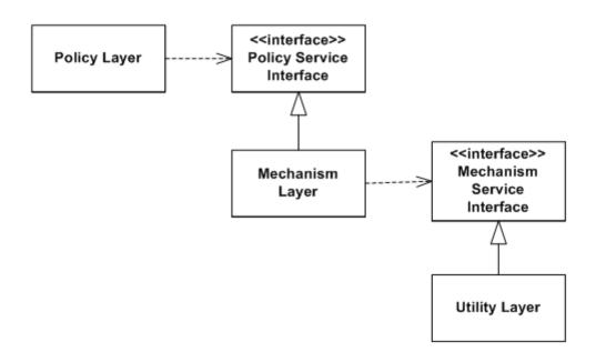
The second part of the principle says, essentially, that high-level modules should not get involved in performing low-level functions.
