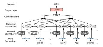
Figure 3: A bidirectional LSTM network for sequence classification.
