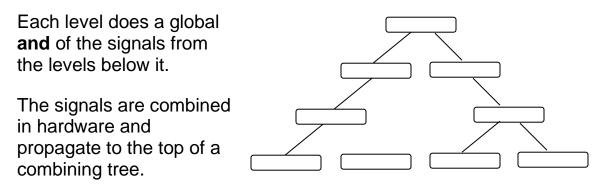
The tree can also be used to do a global interrupt when the entire machine or partition must be stopped as soon as possible "for diagnostic purposes."
