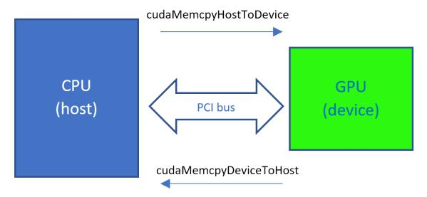
GPUs generally require a host device to activate them. The CPU (host) will run most of the serial code, but for the parallelizable code, it invokes the GPU kernel.
