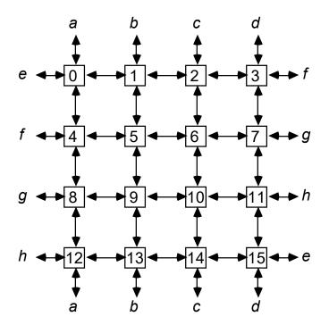
Here is an example of a 16-node mesh. Note that the last element in one row is connected to the first element in the next.
