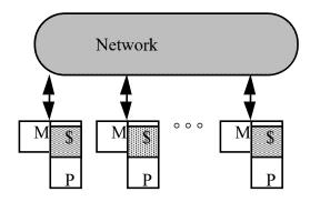
*In shared memory*, the network interface is integrated with the memory controller.
