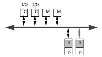
All processors, memories, and I/O controllers are connected to the bus.
