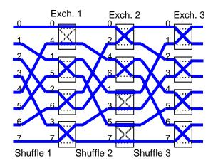
Switches are set to pass through or cross over depending on the exclusive-or of the input and output port numbers.
