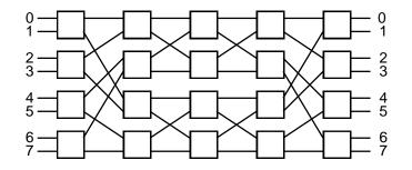
The stages of a Beneš network are connected by shuffle and inverseshuffle permutations.
