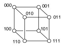
A hypercube is a generalized cube. In a hypercube, there are  $2^n$  nodes, for some *n*. Each node is connected to all other nodes whose numbers differ from it in only one bit position.
