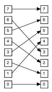
If the links are bidirectional, the *inverse perfect shuffle* is obtained (above, right).
