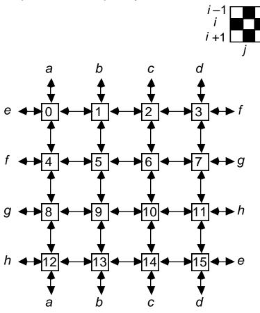
Here is an example of a 16node mesh. Note that the last element in one row is connected to the first element in the next.
