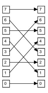
Two variants of the butterfly permutation are the kth sub-butterfly, performed by interchanging bits 0 and k-1 in the binary representation—
